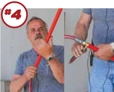
#4 Apply thread-sealing teflon tape to the low pressure swivel end of the foamy brush hose. Thread, by hand, into the brush handle. At this stage, with a wrench, tighten to a snug fit, but do not tighten all the way.
