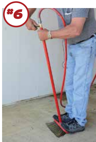
#6 Stand on the brush, gently, and use a wrench to tighten the handle. This also tightens the brush.
