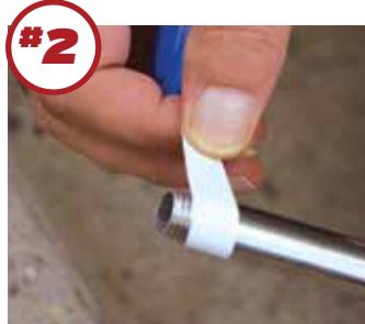
#2 Apply thread-sealing teflon tape to the threading of the new foamy brush hose.
