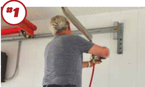
#1 Using two adjustable wrenches, remove the entire foamy brush hose assembly from its connection point at the boom.
